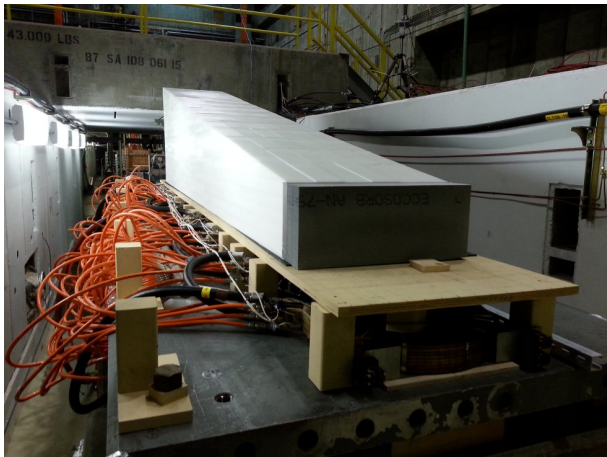
Figure : Electron beam creates secondary cascades in a 4 m long high-density polyethylene (HDPE) target placed in a magnetic field (up to 1000G).
