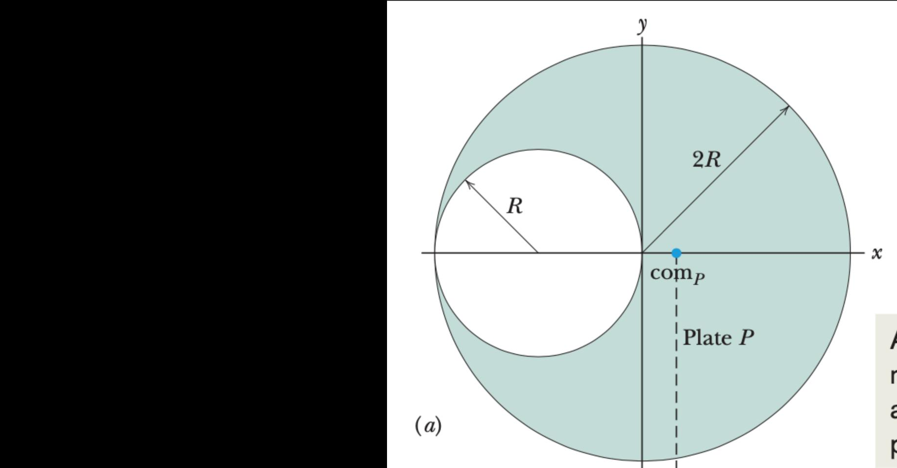
Assume the plate's mass is concentrated as a particle at the plate's center of mass.
