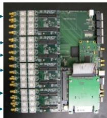
Figure : Each station has 4 string with 16 channels
