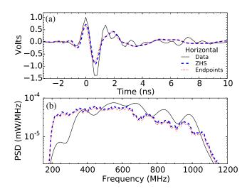
FIG. 2. (a) Simulated and measured voltages 6.52 m above the beam in the horizontal polarization channel at full magnetic field. (b) Corresponding power spectral densities.
