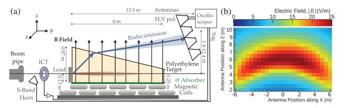
FIG. 1. (a) Schematic of the experiment, not to scale. (b) Simulated (Endpoints) electric field |E| in the x - z plane with full magnetic field, 131 pC, and 4.35 GeV.
