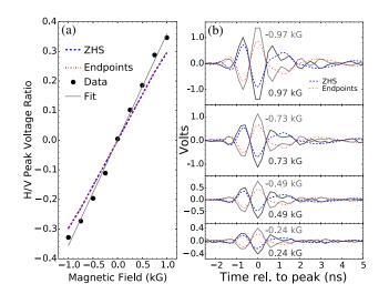
FIG. 3. (a) Horizontally polarized signal normalized by vertical showing the expected linear behavior versus magnetic field. (b) The oscilloscope traces (solid lines) show the polarity flip. Models (dashed lines) are shown for opposite polarities.
